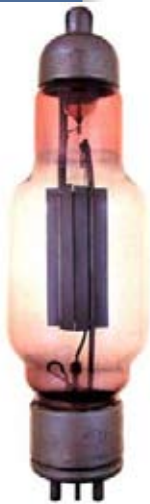
Prototype Gridless Gammatron. Perhaps 5 or 6 known to still exist. (Fig. 1)
