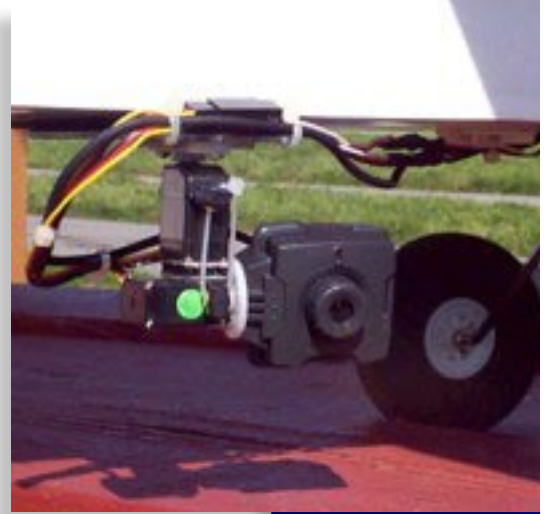
2.4 GHz Camera Mounted Below the Wing of WB4GUK’s R/C Model Airplane
