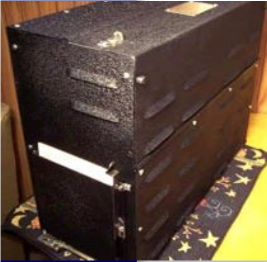
Cabinet Refinished with iBlack Wrinkle Paint
