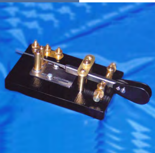
Jeff's Cootie Key (sideswiper), built by Joe Medsker, K8LKC
