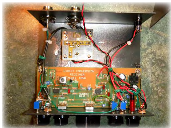
Ten Tec Receiver PCB in Enclosure
