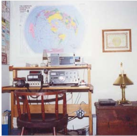
Early 1990, Station shared by NIØC and son AAØBP (apartment QTH in Kirkwood, Mo.), showing Kenwood TS-520S transceiver, Sony 2010 receiver (used for wide splits in DX pileups), and MFJ Grandmaster keyer with Vibroplex Vibro-keyer paddle. NIØC made the first CW QSO with the 1990 3D2AM Conway Reef expedition using this station.
