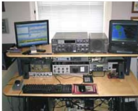
Fast forward to 2008. ARS NIØC using Ten Tec Omni VI, Elecraft K2, Kenwood TS-930S, Ameritron Amplifier, MFJ DSP, computers, top-loaded Butternut HF-2V, Force 12 Sigma-40 vertical antenna and more!
