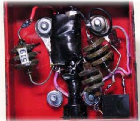
RF Filters Installed in Base of Paddle
