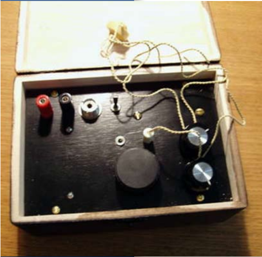
Exterior View of Finished Receiver
