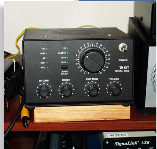
Ten-Tec 1253 Regenerative Receiver Kit
