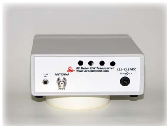
Rear Panel View of Completed Ft. Tuthill 80 Transceiver
