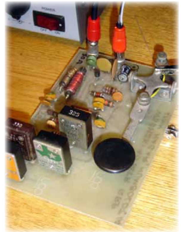
40-meter XMTR; 300 mW
