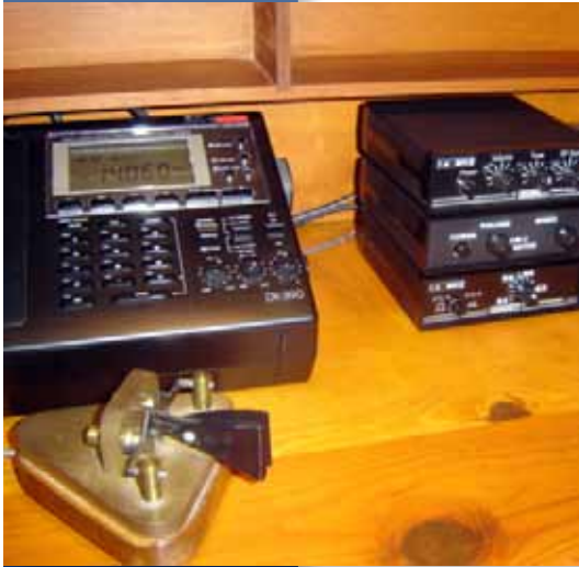
20-meter Station in Roll-Top Desk; 750 mW
