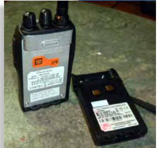
Rear View with Li-ion Battery Removed
