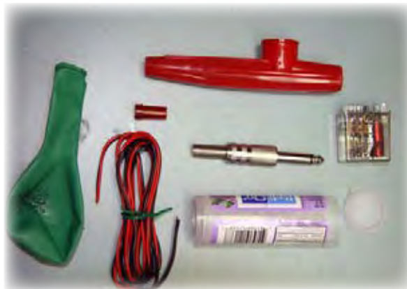
The Parts that go into a W5IG Air Key
